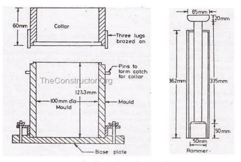
standard proctor test apparatus
