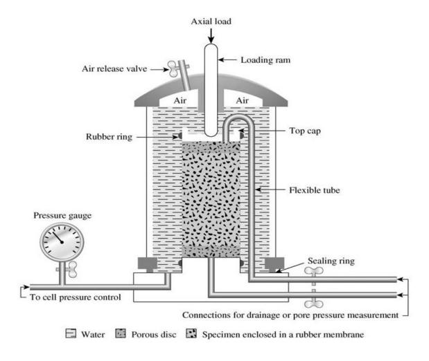
Diagram of triaxial test equipment
