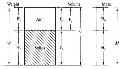
Block diagram - phases of a Dry soil element
