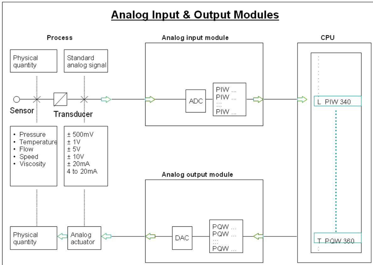
Fig.5 Analog I/O Modules
