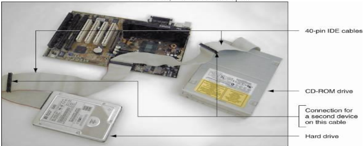
Two IDE devices connected to a motherboard using both IDE connections and two cables
