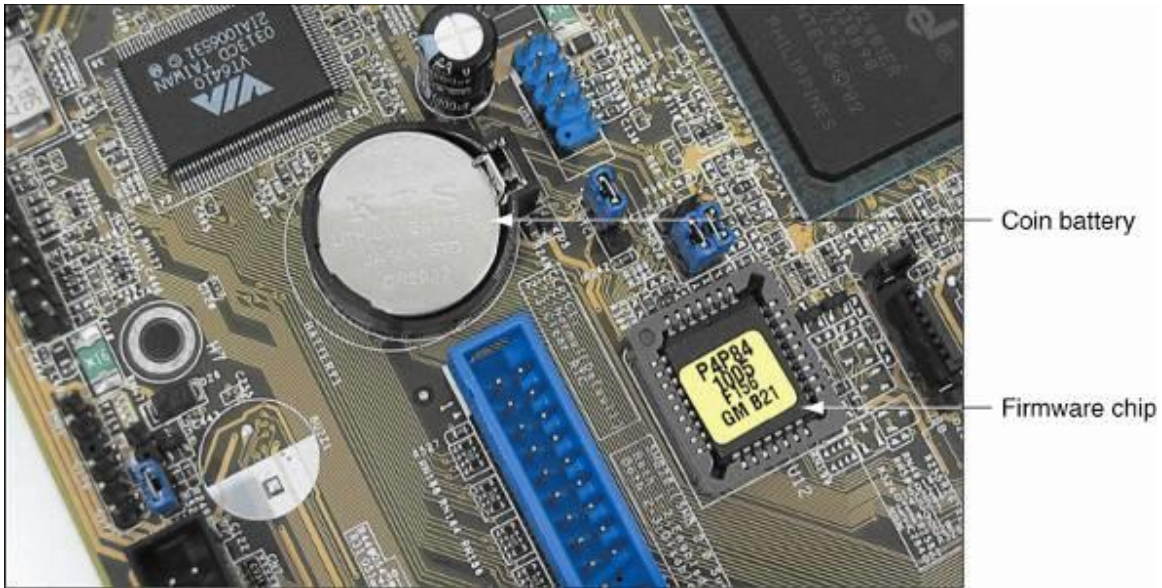
This firmware chip contains flash ROM and CMOS RAM; CMOS RAM is powered by the coin battery located near the chip
