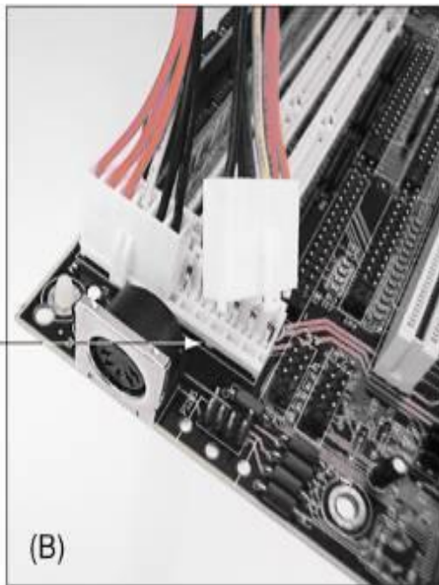
Power connectors on a motherboard
