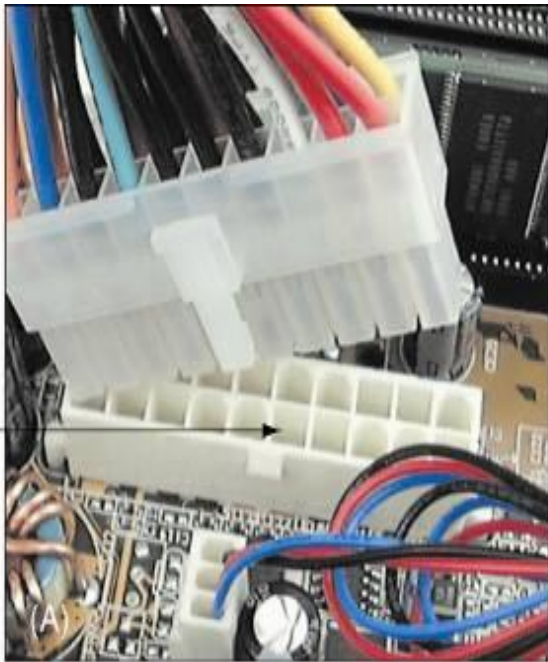
P1 power connector on a motherboard
