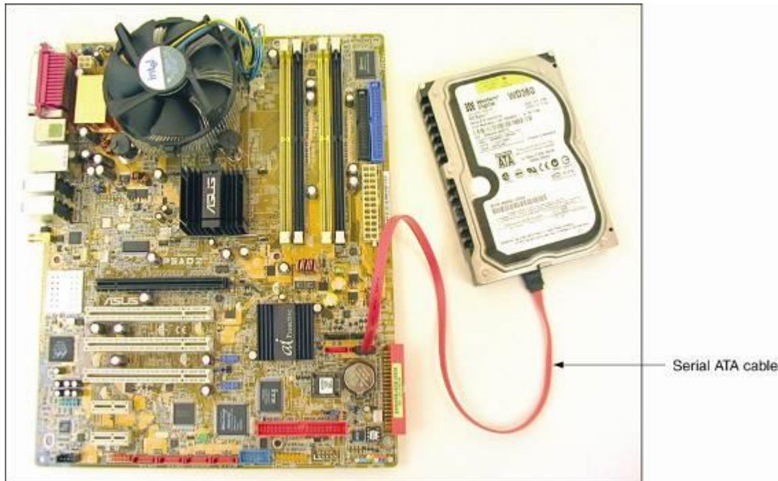
A hard drive subsystem using the new serial ATA data cable
