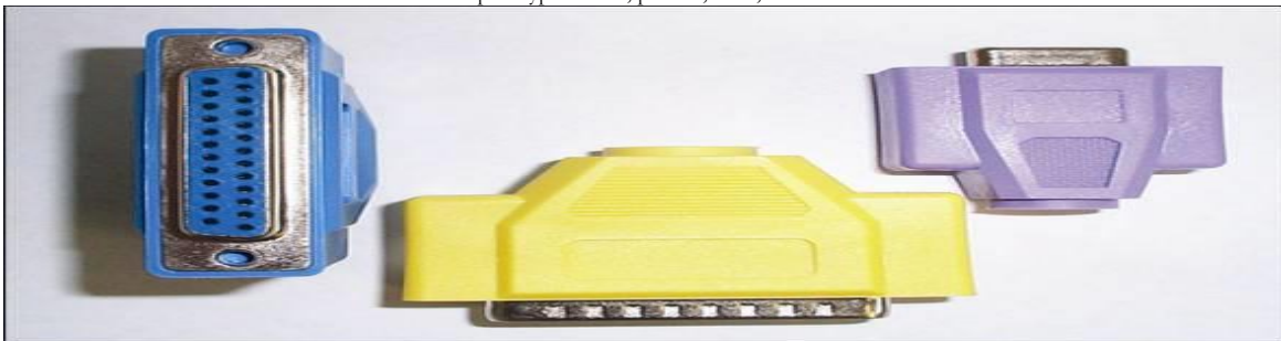
Loop-back plugs used to test serial and parallel ports
