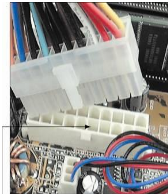
P1 power connector on a motherboard
