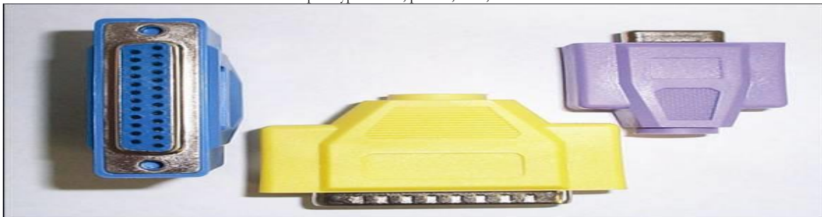
Loop-back plugs used to test serial and parallel ports
