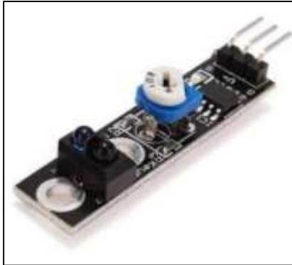
Fig 36. Line Follow Sensor Module
