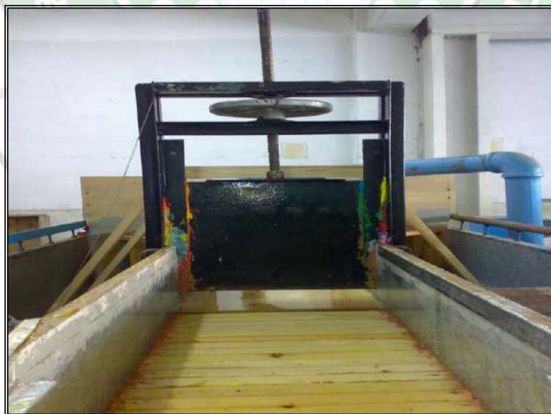
Plate (1): Crests of corrugations are at the same level of the upstream bed
