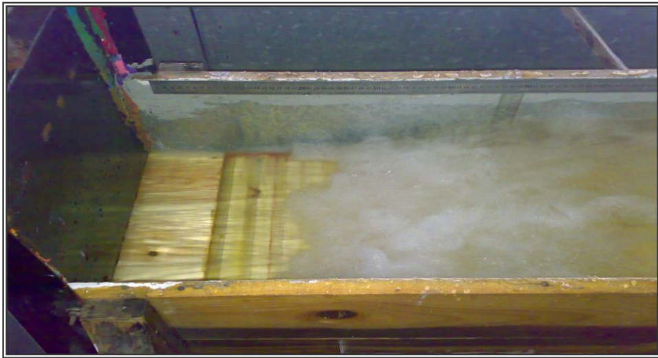
Plate (2): Steady jump ( Fr=5.6 ) over triangular corrugated bed
